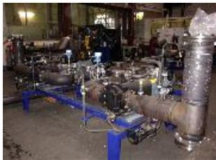
Up to the time of adding the finished polymer mix to the production process by means of the discharge pumps (Fig. 11), the mixing vessel functions as a storage tank for the production.
