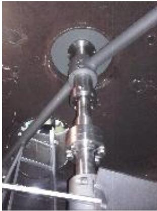
The mixing vessel has been equipped with a coaxial agitator mixing the mass in several stages (Fig. 09). To prevent detrimental emissions entering the environment, the entire equipment operates with an environmentally friendly gas displacement system. When the mixing vessel is filled, the gas is pressed out of the vessel. This is conveyed back into the discharge container, the raw-material storage tank.
