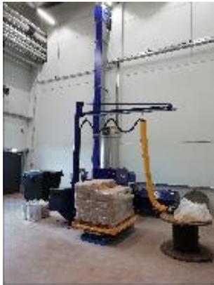
Resin ingredients are delivered as small flakes, just about in finger-nail-size, packed in sacks. First, the flakes are loaded into a collecting tank. As the resin flakes easily stick together, the Keil engineers installed a bucket conveyor system (Fig. 06) for a smooth transport into the mixing vessel.
